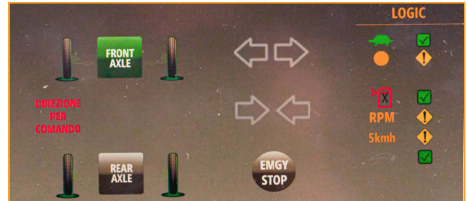
Option Automatic Open/close Axle from cabin, directly from TERA monitor Intermediate position available by fixing bracket
