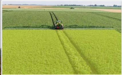
Concentrated start with pressure circulation
