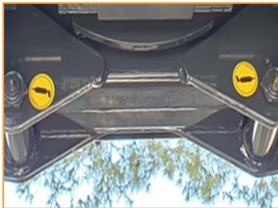
Anti-friction rollers to keep axle adjustments easier!
